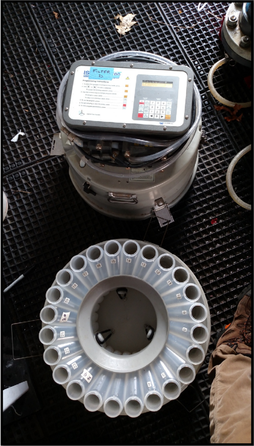
Figure 2.08: Autosampler Programmed for Collecting Grab Samples
