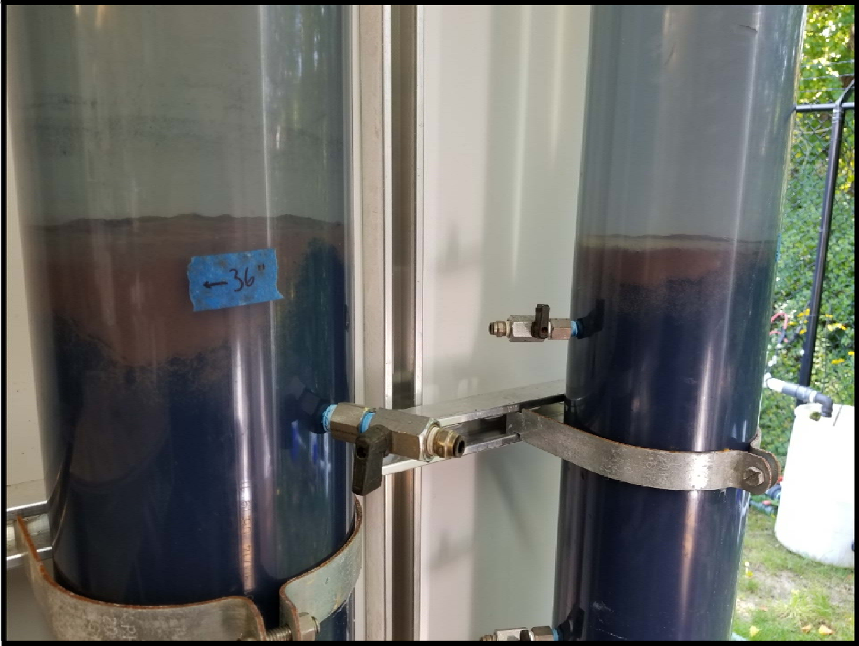
Figure 4.12: Iron Accumulation on the GAC Contactor Media Surface
