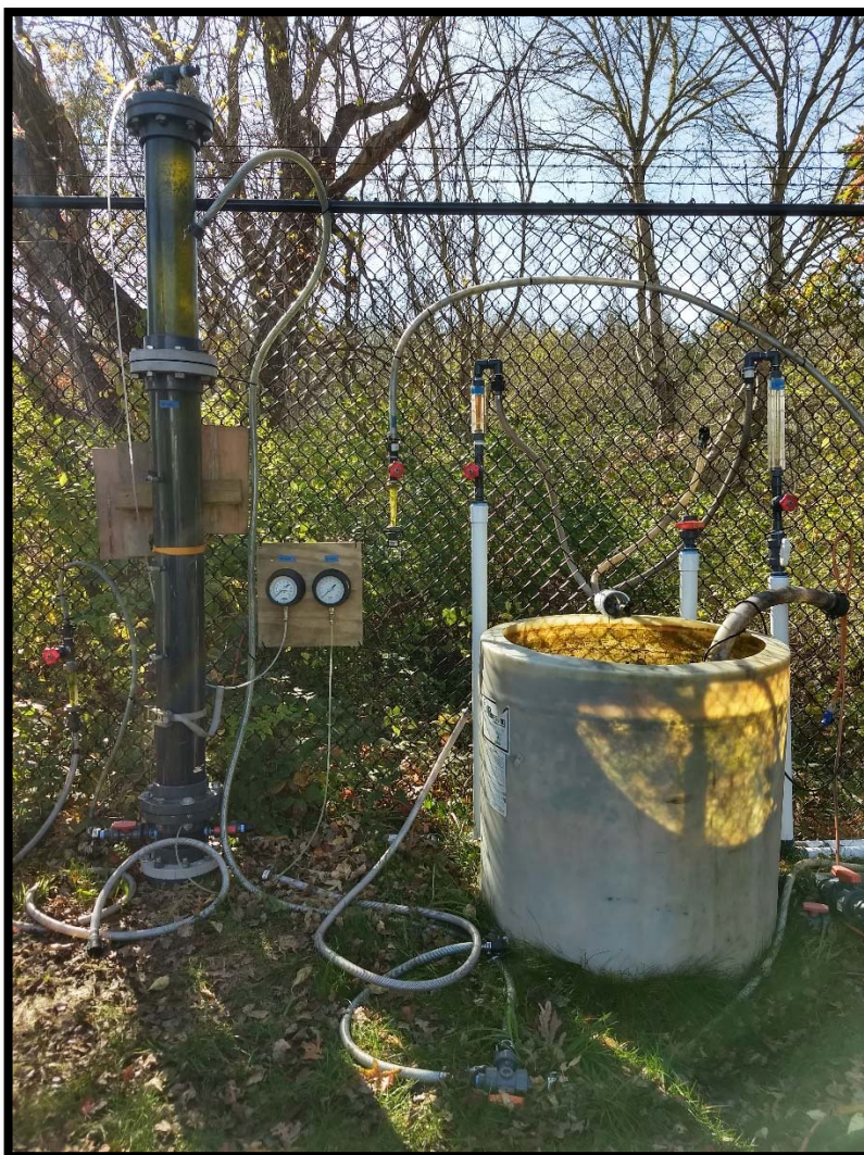
Figure 1: Pilot Scale GAC Contactor and Blending Tank
